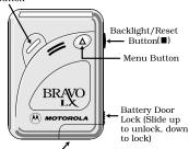
Slide battery door to the right (Insert positive end of battery first) ACPB-952424-0
